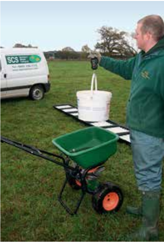
SCS Spreader & Sprayer Testing is the UK's largest independent fertiliser spreader testing specialist and their advice to operators is to ensure equipment is properly maintained and tested for application rate and distribution pattern with every product it will apply. Spinning disc spreaders will also need to be tested over trays to determine the true spreading width and evenness of distribution.
